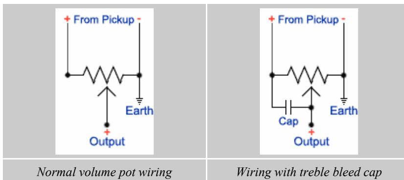
**How to do It:** Simply solder a capacitor from the live terminal on your volume pot (where the wire from the selector switch attaches) to the centre wiper terminal. When the volume is up full, this cap has no effect on the tone, but as the volume is turned down, more treble frequencies are bled
